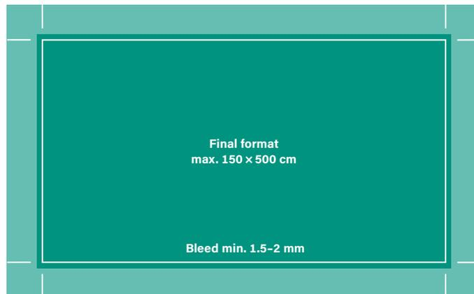
**Fig. 1** Bleed for mountings onto panels
